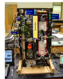
Cloud Condensation Nuclei Counter, US Patent 7,656,510
